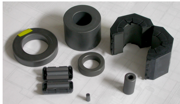
Fig 5 – Ferrites are made in many forms
