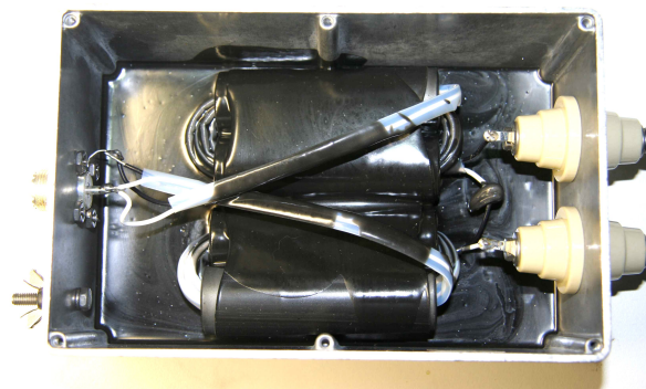
Fig 38 –Choke (Guanella) Transformer
